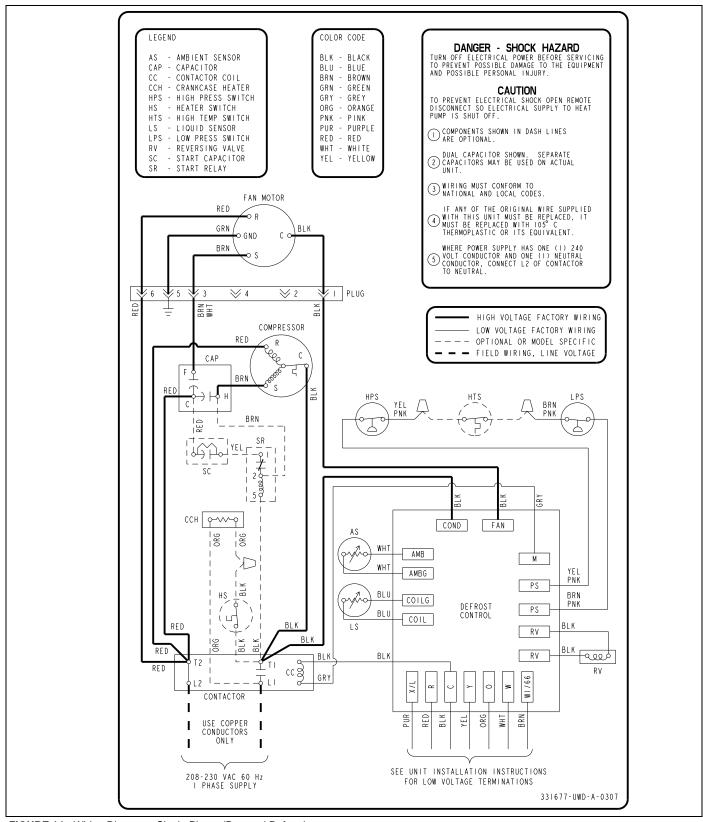
FIGURE 14: Wiring Diagram - Single Phase (Demand Defrost)
