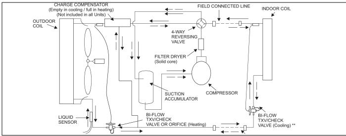
FIGURE 10: Heat Pump Flow Diagram
