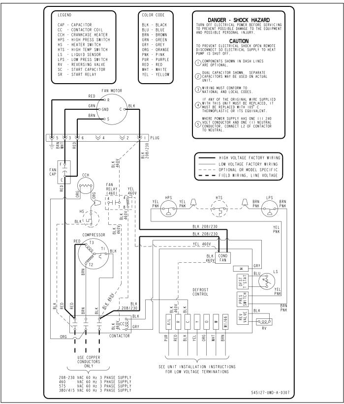
FIGURE 17: Wiring Diagram - Three Phase (Time-Temp)
