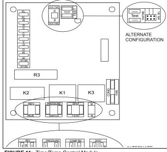
FIGURE 11: Time/Temp Control Module
