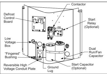
FIGURE 6: Outdoor Unit Control Box - Single Phase
