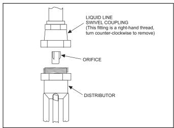
FIGURE 5: Orifice Installation
