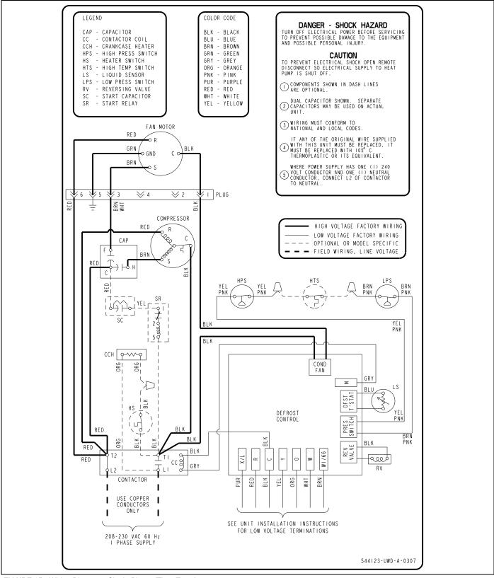
FIGURE 15: Wiring Diagram - Single Phase (Time-Temp)
