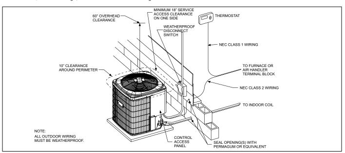
FIGURE 1: Typical Installation with Required Clearances
